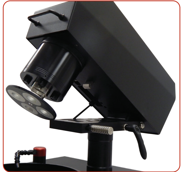
Unique tilt-up feature allows easy access to platen and holder.
