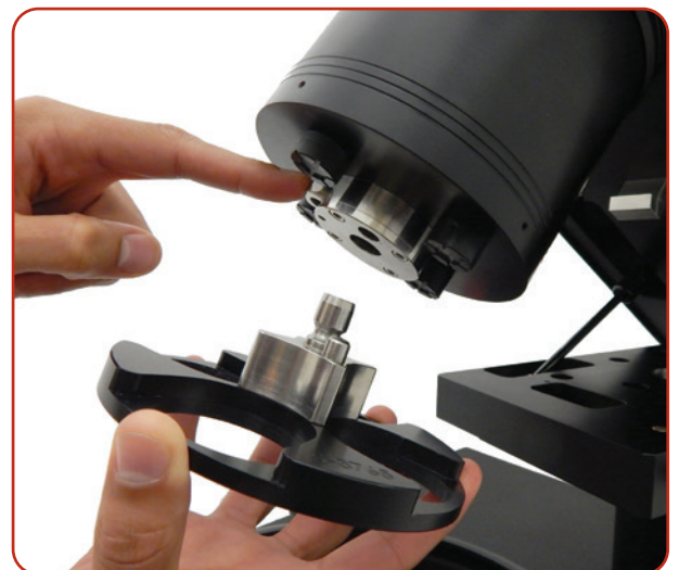
Simple push-button allows easy attachment and removal of sample holders.
